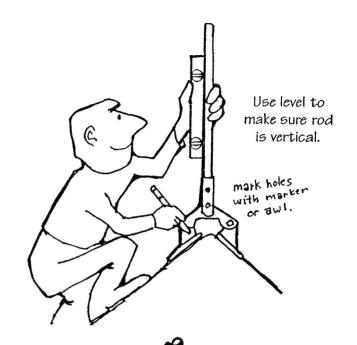
Check rod for plumb (use level). Drill 3/32" holes using roof mount as template. Fill holes with caulk and drive in 2" screws supplied.
